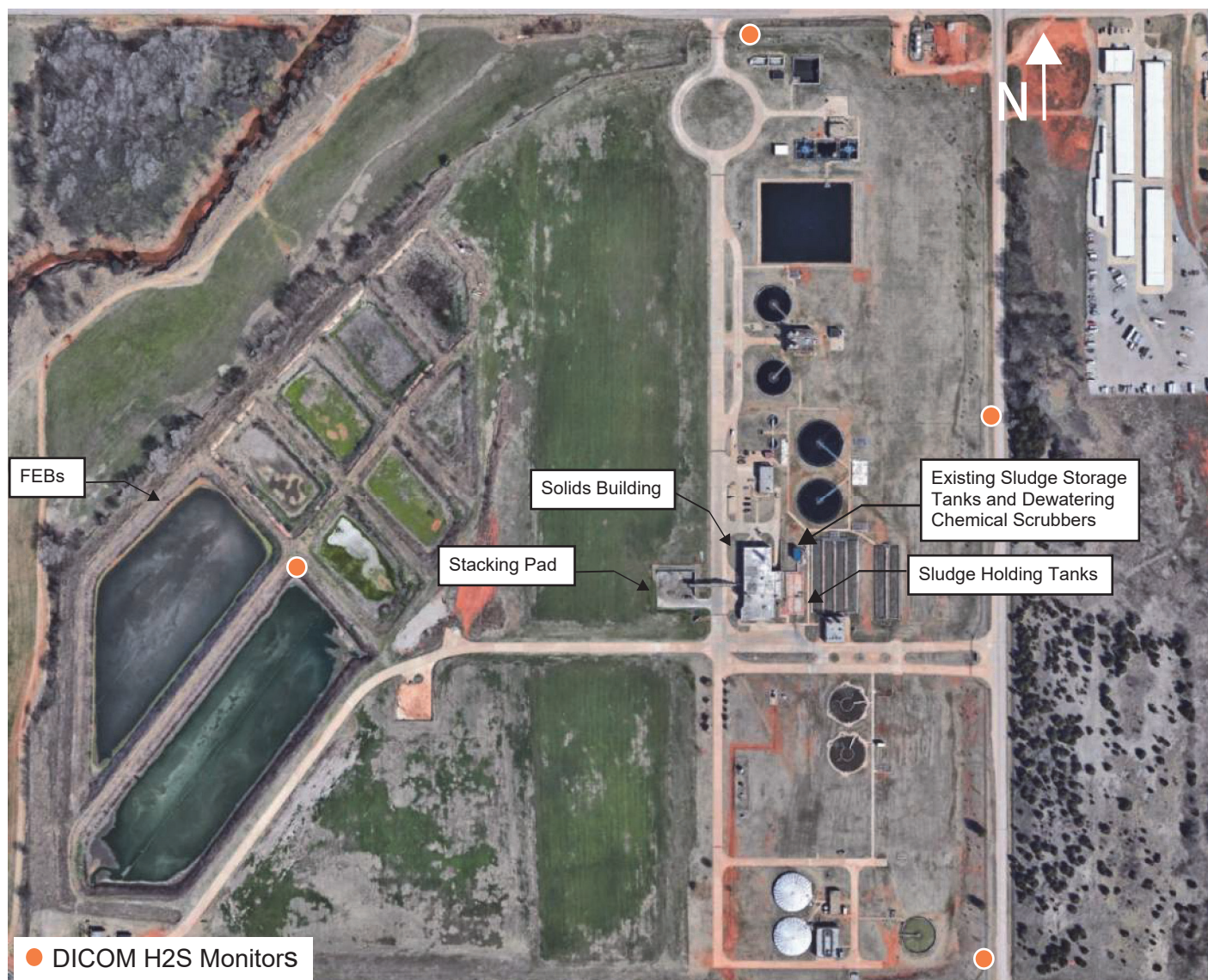
Proposed locations for DICOM H 2 S monitors at Deer Creek WWTP
