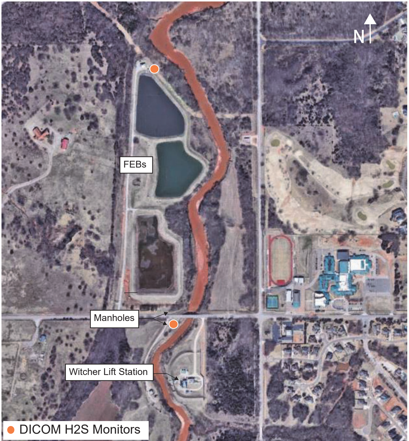
Proposed locations for DICOM H2S monitors at Witcher Lift Station
